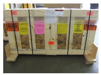
Remove 4 perimeter screws from face lid noted as "OPEN THIS SIDE." Remove face lid.
